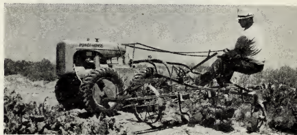
Eimco Power-Horse attached to "horse-drawn" cultivator making turn at end of row in a field of sugar beets. Turning space required is less than the width of the cultivator. Operator has perfect control of both Power-Horse and cultivator—can accomplish at least three times as much work in a day as with a team.
