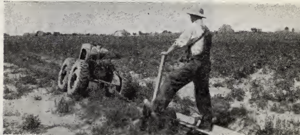
Try to do this ditching job with any two-wheel-drive tractor! Only the positive four-wheel drive of the Power-Horse can give adequate traction with two wheels in the muddy ditch.
