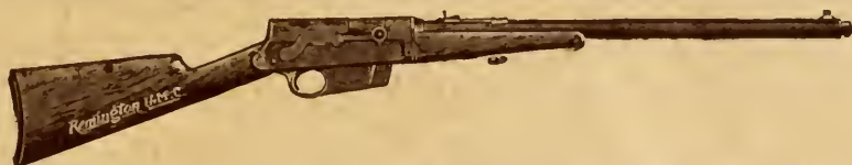
REMINGTON AUTOLOADING RIFLE—ONE OF BROWNING'S PATENTS
