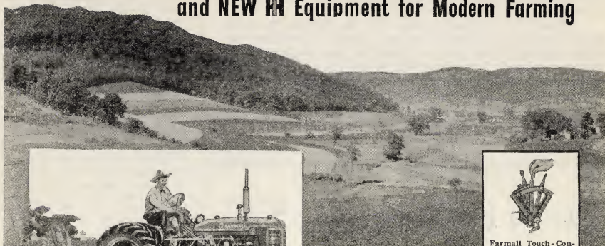
Farmall Touch-Control is a complete implement control. Hydraulic power in both directions—power to lift implement from the ground and force it into the ground.
